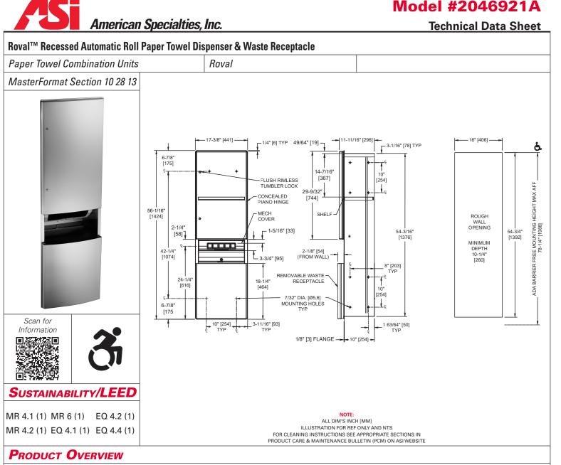
Proximity sensing no-touch unit dispenses a pre-set length per cycle from 8" [205] or 9" [230] wide standard towel roll up to 800 ft. (244m) long and has stub roll capability for continuous dispensing. Smaller waste receptacle, 13.5 gal. (51.1 L), allows unit to be ADA compliant. Internal shelf is ideal for paper towel storage. Towel length is determined by owner by setting length, delay and paper saver switches. Powered by 4 D-size batteries (not included).
