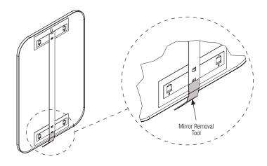
**Models 7B1-10XXXX and 7B1-30XXXX:** While holding the handle side of the mirror removal tool in one hand, insert the removal tool through the bottom center opening in the mirror shelf and then place the working end of the tool between the mirror and shelf.
